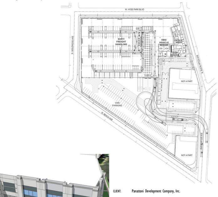
DESCRIPTION: The project consists of a 143,600 square feet building that includes a 9,300 square feet Office/Ship Center tenant improvement, 2,700 square feet Vehicle Maintenance, and a 131,600 square feet Sort/Freight Area serving 108 drive-in van positions. The building also features a 32' clear height
